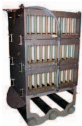
Ceramic membrane filtration units with three filter modules, Photo: Bergmann Umwelttechnik
